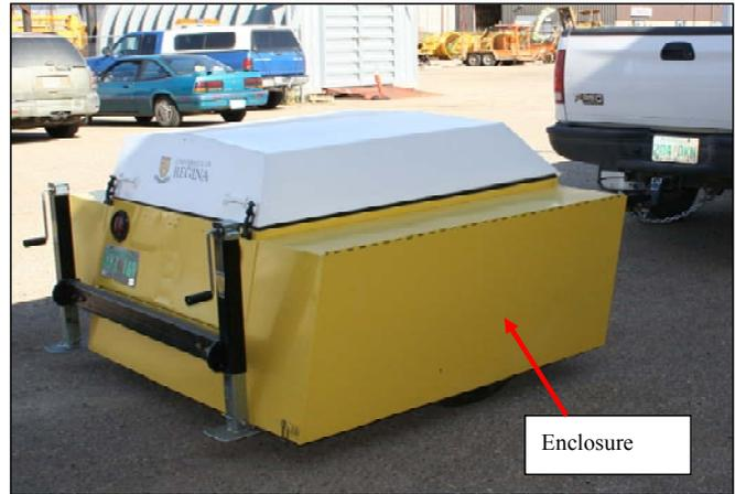
Figure 2. CPX test trailer.
