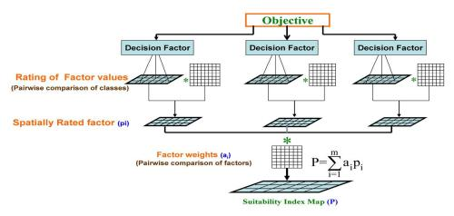
Figure 6. Conceptual implementation of spatial analytical hierarchical process.
