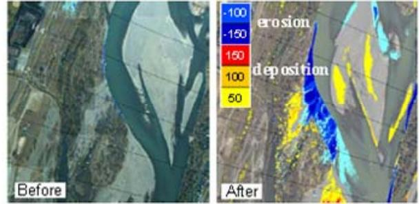
**Figure 5.** High-vegetation related bank erosion site.
