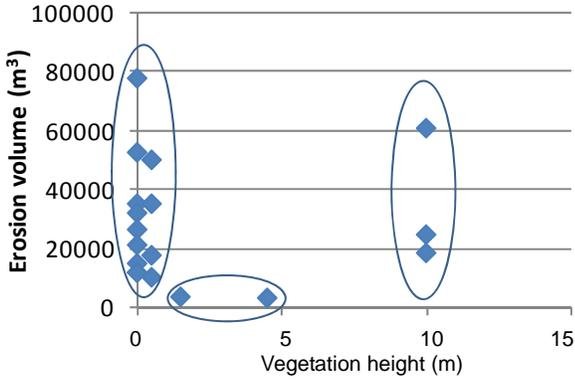
**Figure 4.** Relation between vegetation height and erosion volume.
