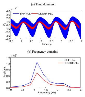
Figure 8. Performance of different PLLs in the power system under single-phase break. (a) Time domains; (b) Frequency domains.
