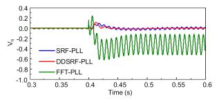
**Figure 5.** Performance of different PLLs after a step change in amplitude and phase of the phase-A voltage.
