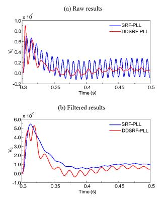
**Figure 10.** Performance of different PLLs in the power system under line-to-line ground short circuit. (a) Raw results; (b) Filtered results.
