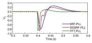
**Figure 4.** Performance of different PLLs after a step phase decrease of the three-phase voltage.
