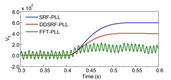
Figure 12. Performance of different PLLs considering power system dynamics and first-swing stability.
