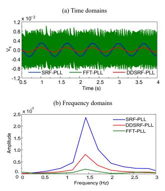
Figure 7. Performance of different PLLs in the power system under load shedding. (a) Time domains; (b) Frequency domains.
