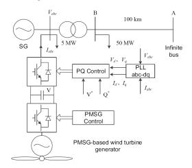
Figure 6. Structure of a power system to evaluate PLL performance (PMSG, permanent-magnet SG).
