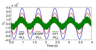
Figure 11. Performance of different PLLs considering power system dynamics under low-frequency oscillation.
