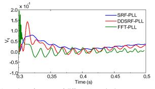
**Figure 9.** Performance of different PLLs in the power system under three-phase-to-ground short circuit.
