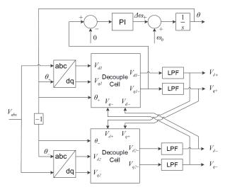
Figure 2. Structure of DDSRF-PLL.
