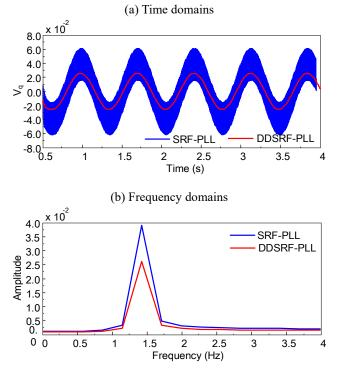
**Figure 13.** Performance of different PLLs considering power system dynamics under low-frequency oscillation and unbalanced operation. (a) Time domains; (b) Frequency domains.
