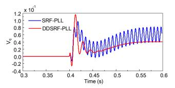
Figure 14. Performance of different PLLs considering power system dynamics and first-swing stability under unbalanced operation.
