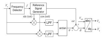
Figure 3. Structure of FFT-PLL.
