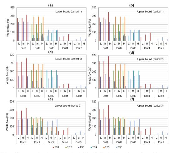
Figure 1. Wastes shipped to transfer stations under case 1. (Symbols of "L, M and H" denote "low, medium and high waste-generation levels", respectively; "Dist" and "TS" are abbreviations of "district" and "transfer station", respectively)
