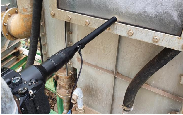
Figure 4. Bubble-image extraction in the atomizer using a DSLR camera.
