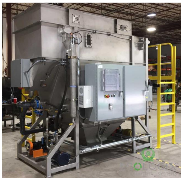
Figure 5. DAF system developed by Ecologix Systems. Reprinted from Ecologix Environmental Systems (2022).
